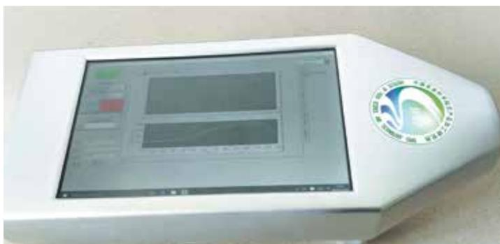
▲ Non-destructive near-infrared grading equipment for sheep carcass
